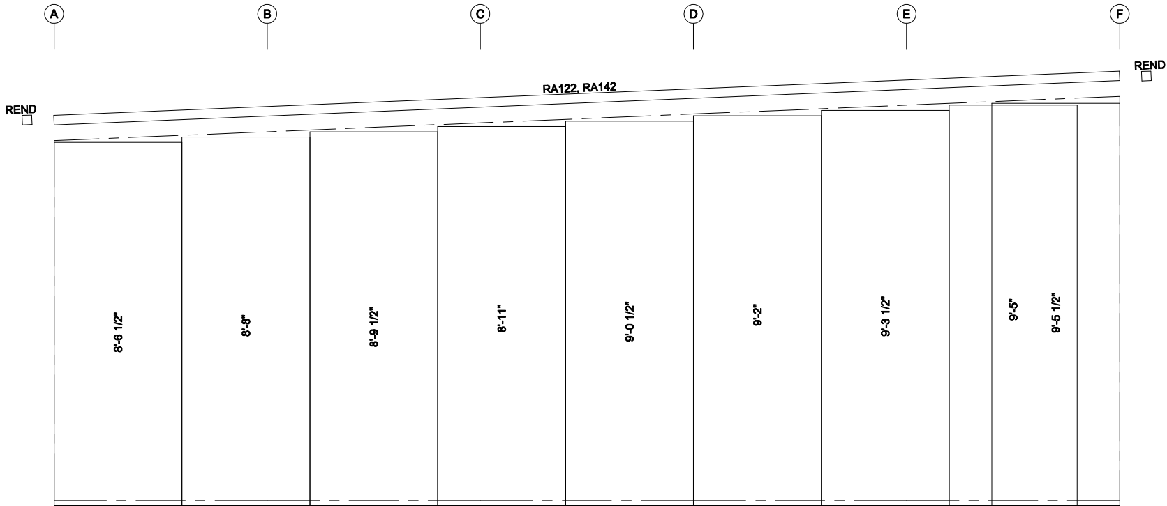
ENDWALL SHEETING & TRIM FRAME LINE: 1
