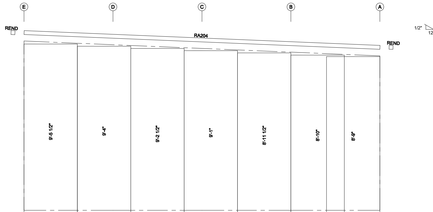
ENDWALL SHEETING & TRIM FRAME LINE: 18
