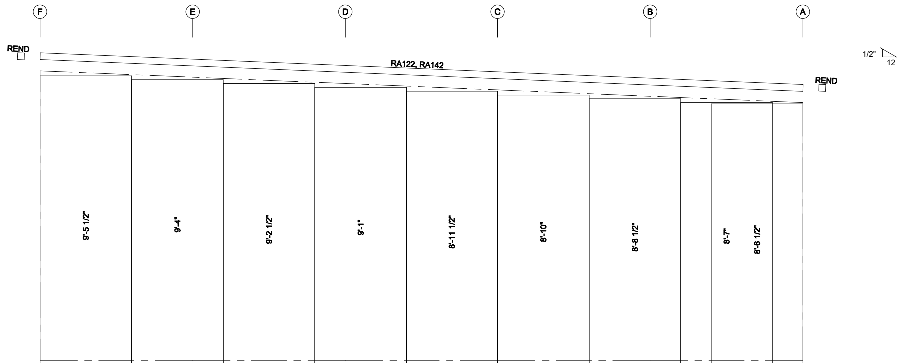
ENDWALL SHEETING & TRIM FRAME LINE: 17
