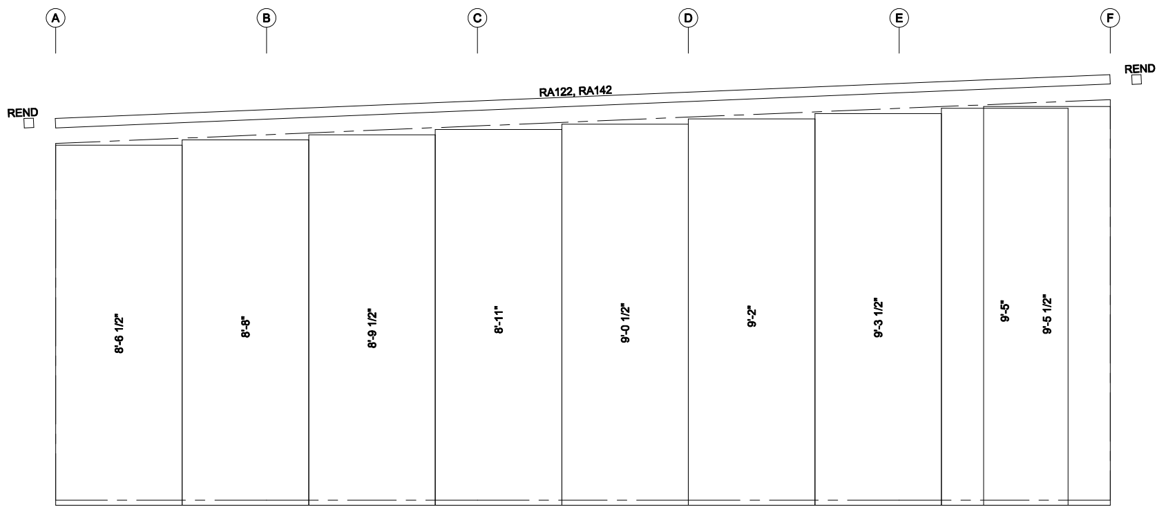
ENDWALL SHEETING & TRIM FRAME LINE: 1
